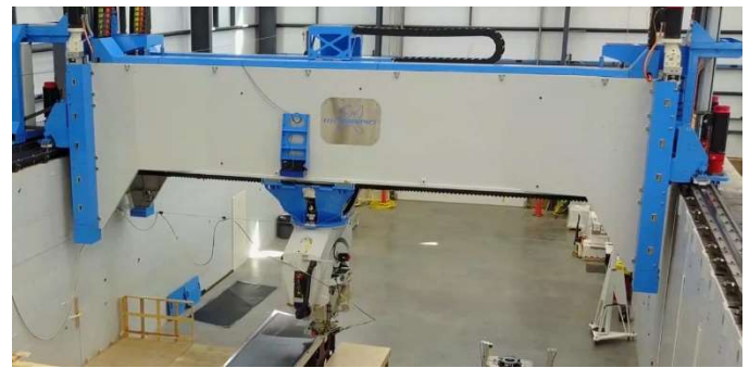
Figure 6. High Performance AFP gantry machine.
