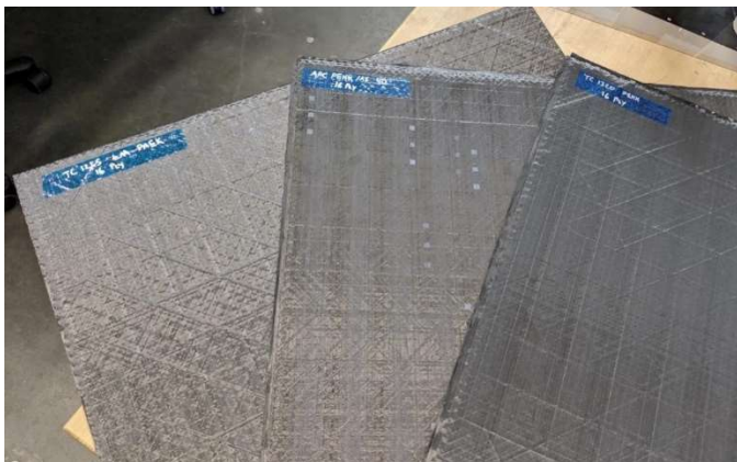
Figure 16. Quilting patterns emerge as more plies are laid down. The effect is exaggerated to unacceptable levels at high speeds.
