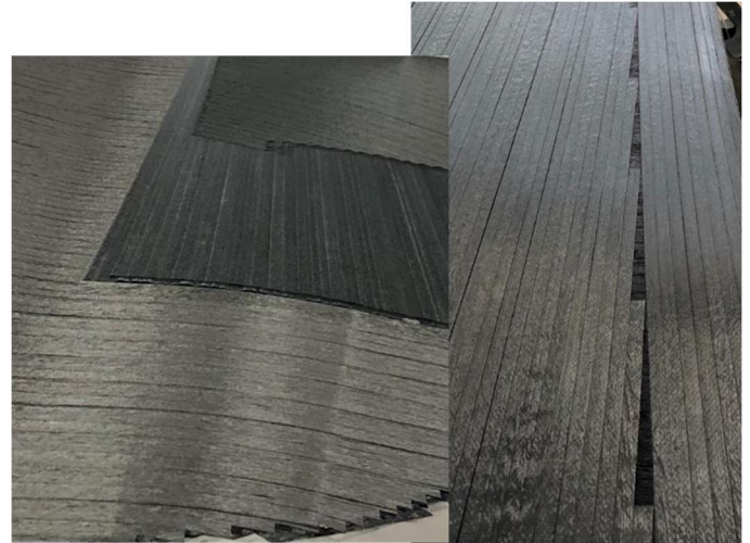
Figure 3. Part lamination features (pad-ups to the left and convergent zones to the right) that contain interior tow ends or drops.
