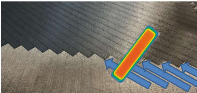
Figure 2. Fixed Spot Size Laser does not accommodate variable number tows.
